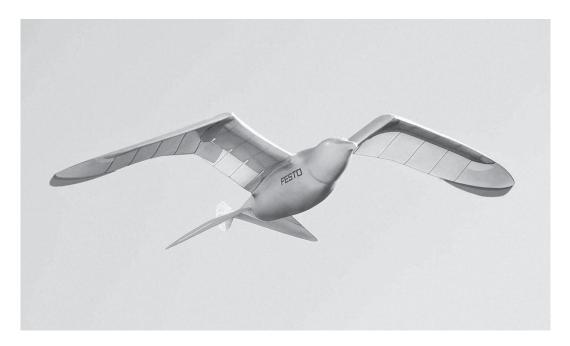
and automation company based in Esslingen am Neckar. The laboratory specializes in lightweight material and advanced pneumatics. The movements of the bird have been precisely engineered to match the patterns of a seagull. They are exploring what they call "bionic thinking" and their goal is to "learn from nature and transfer that knowledge into technology to improve the production of the future." But to what end?
